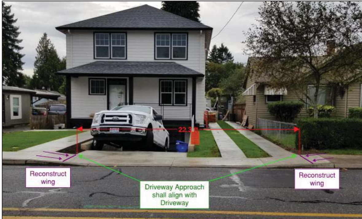
Figure 6. Street-view illustration of recommended conditions of approval with variance for increased driveway width – Option A.
