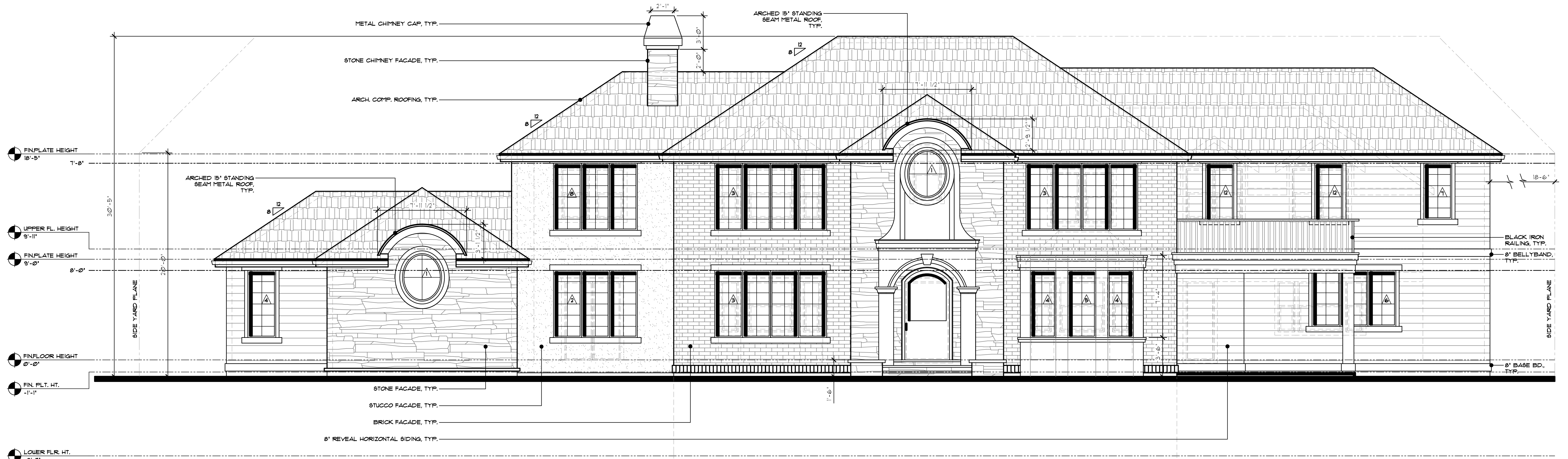
FRONT ELEVATION 5,236 SQ. FT. EXISTING RESIDENCE 1,184 SQ. FT. NEW ADDITION 1,020 SQ. FT. TOTAL
