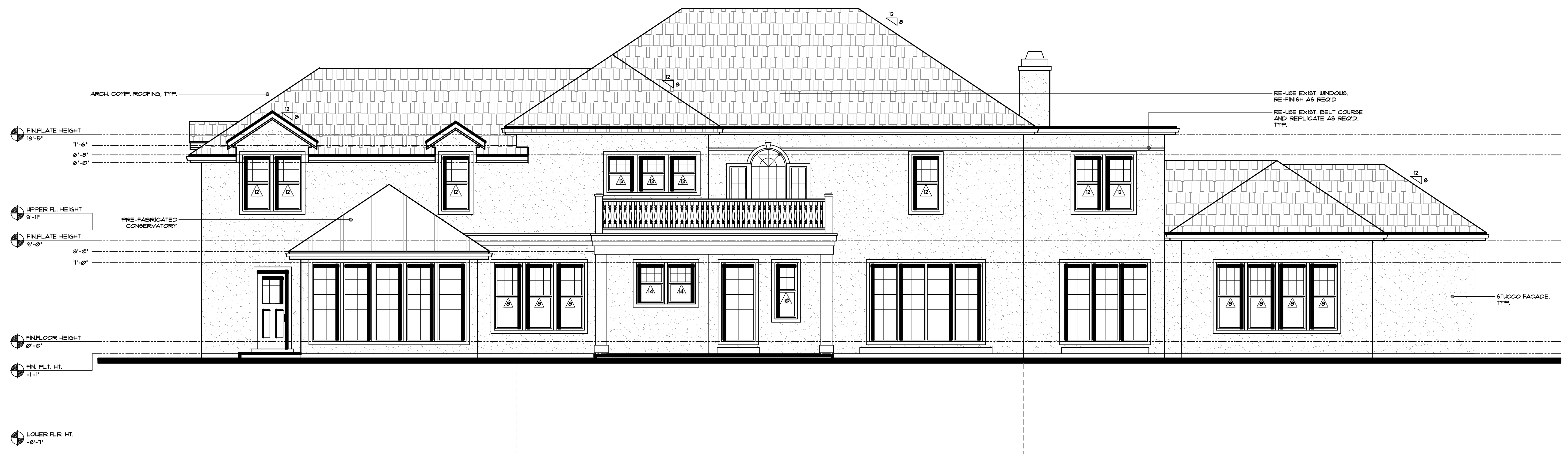
REAR ELEVATION 5,236 SQ. FT. EXISTING RESIDENCE 1,784 SQ. FT. NEW ADDITION 7,020 SQ. FT. TOTAL
