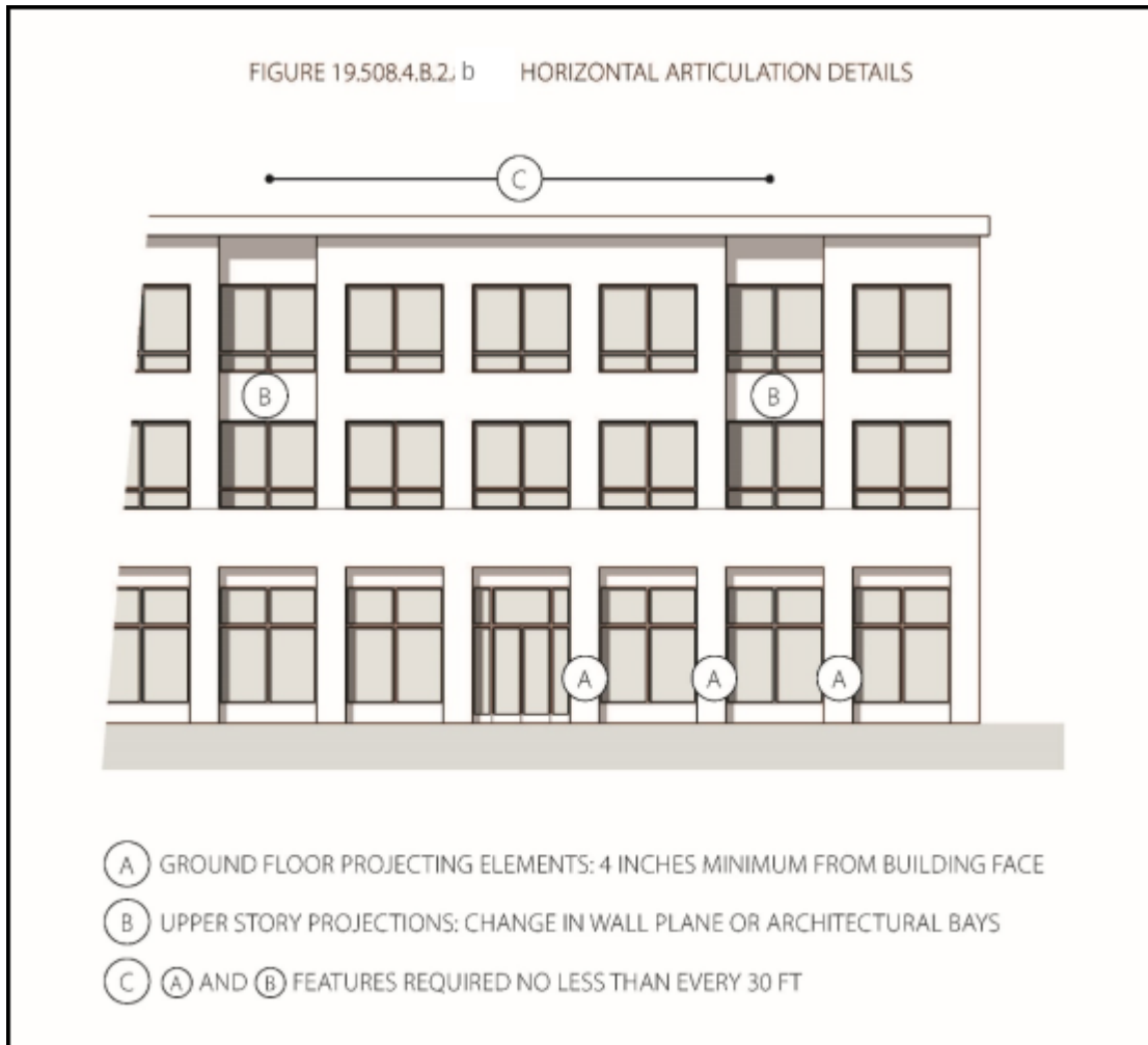
Figure 19.508.4.B.2.b Horizontal Articulation Details
