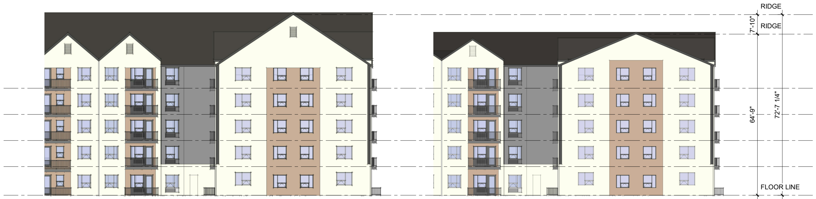
END ELEVATION WITH 8:12 MAIN ROOF PITCH
