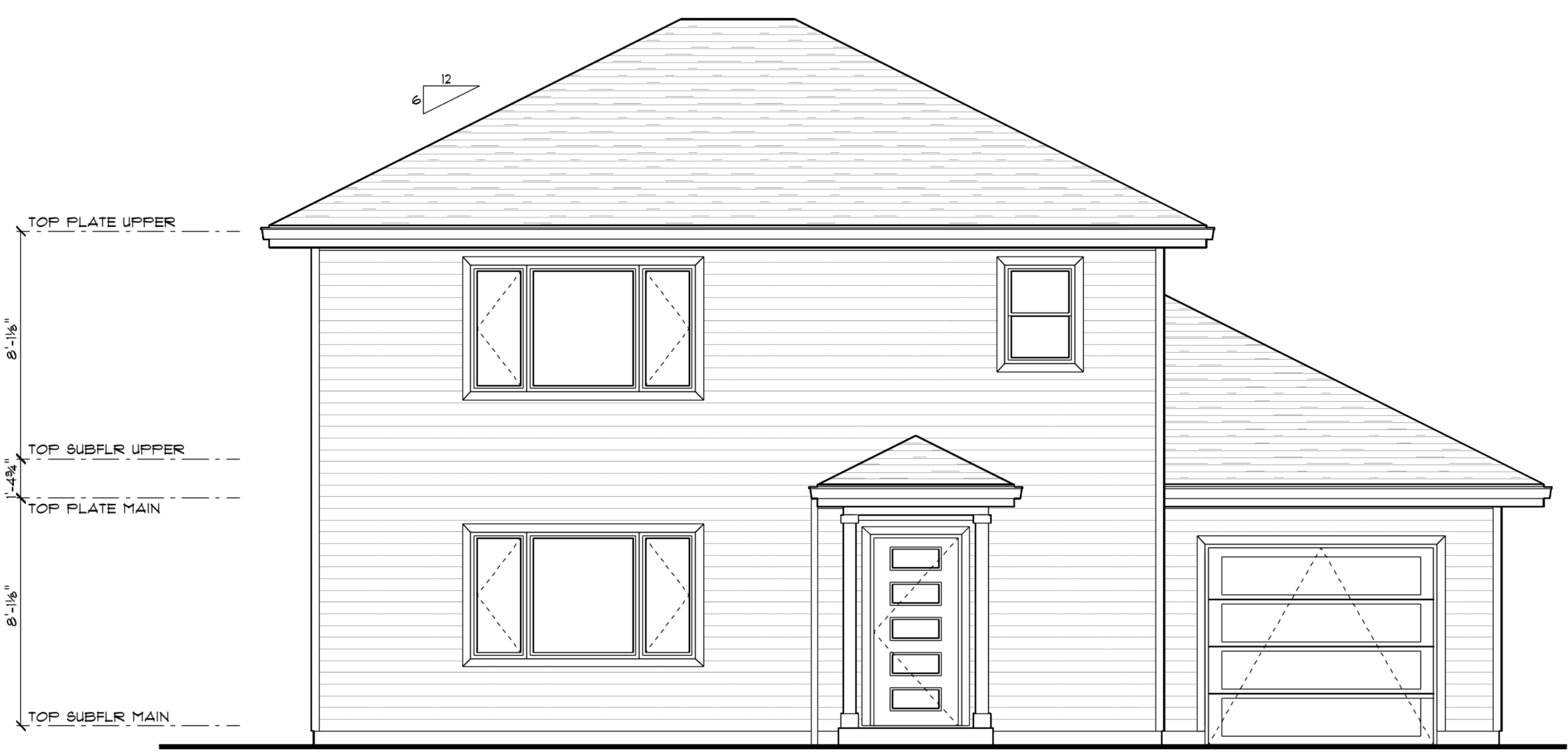
FRONT ELEVATION SCALE: 1/4" = 1'-0"
