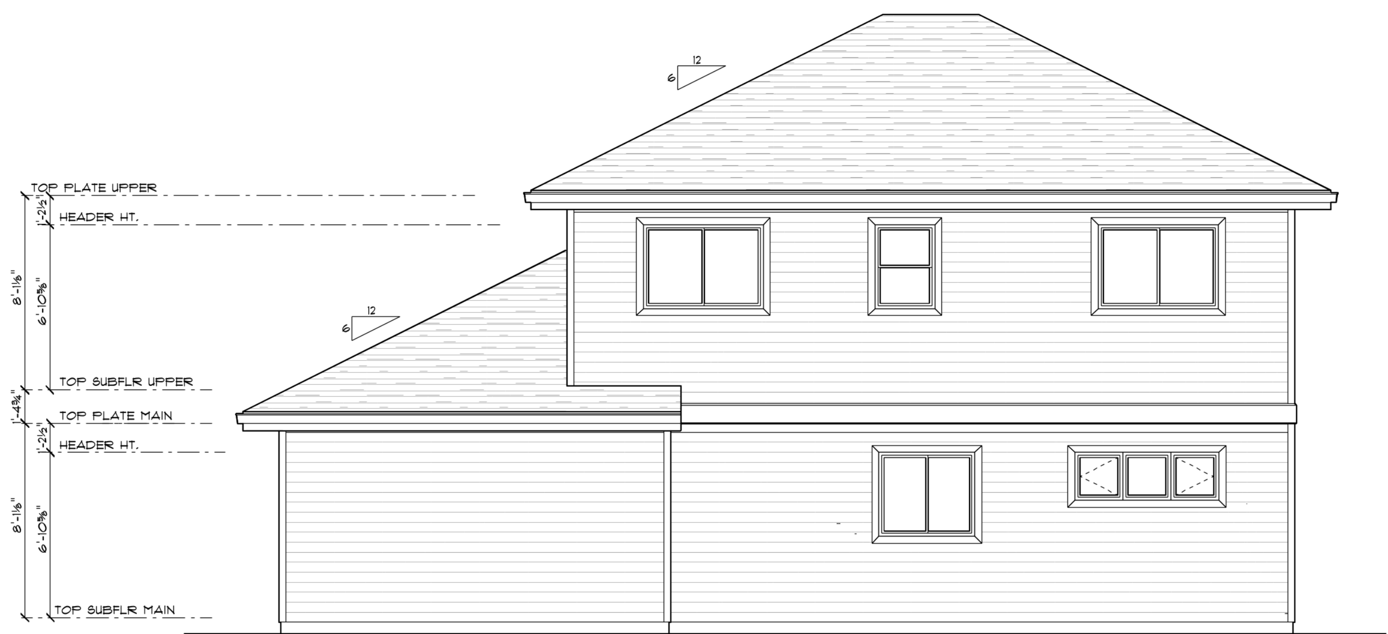
REAR ELEVATION SCALE: 1/4" = 1'-0"
