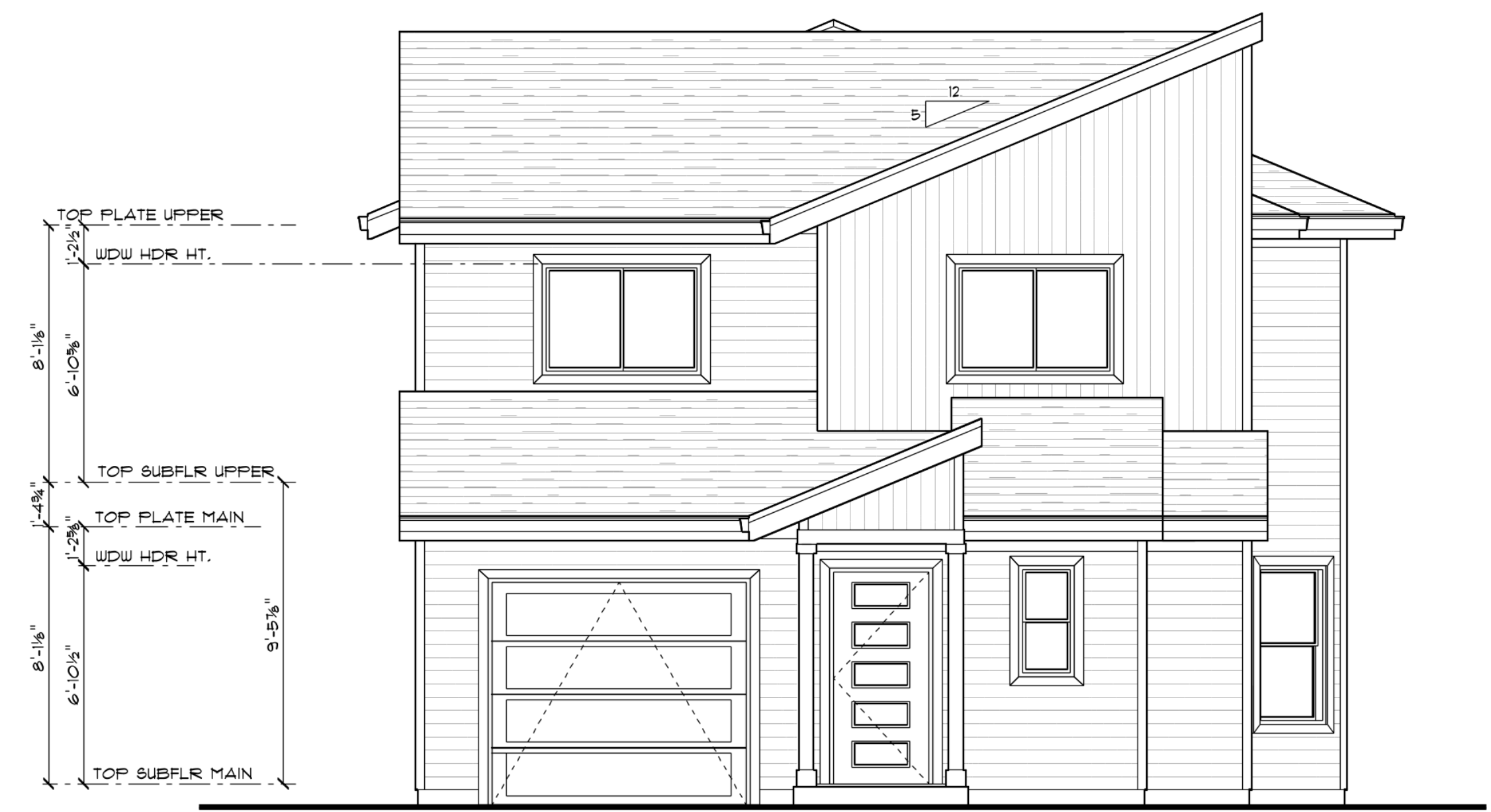
FRONT ELEVATION SCALE: 1/4" = 1'-0"
