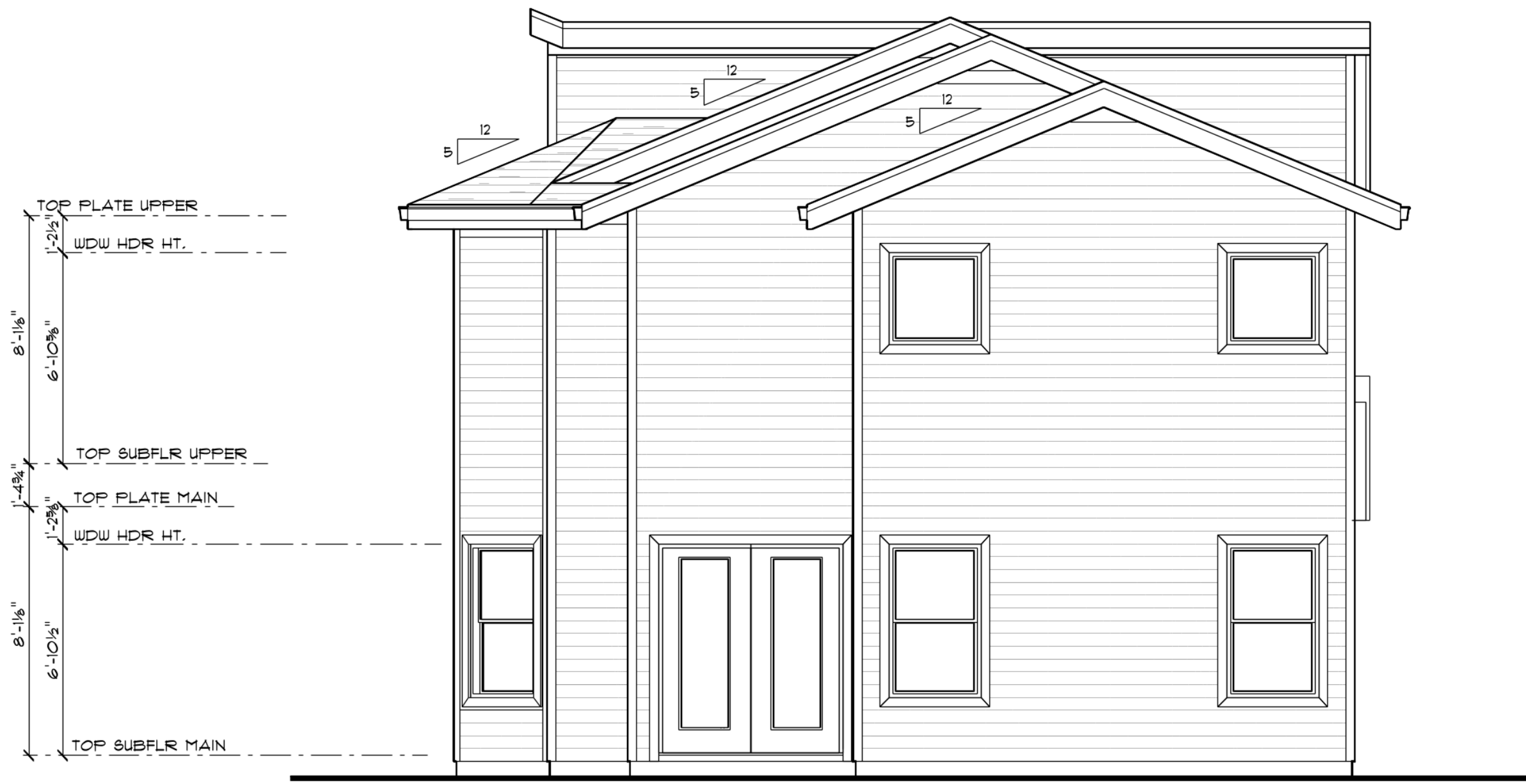
REAR ELEVATION SCALE: 1/4" = 1'-0"
