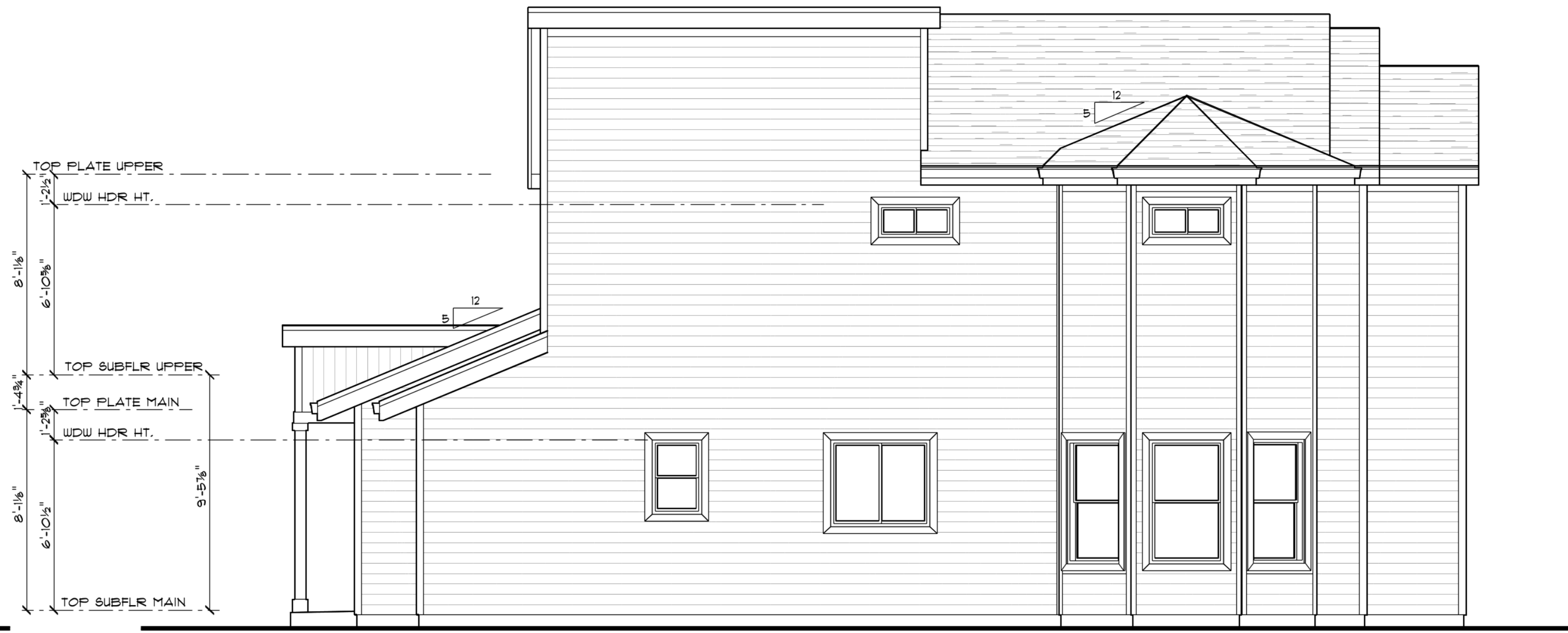
RIGHT SIDE ELEVATION SCALE: 1/4" = 1'-0"
