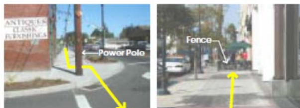
Not Recommended: Indirect pedestrian routes with obstructions
