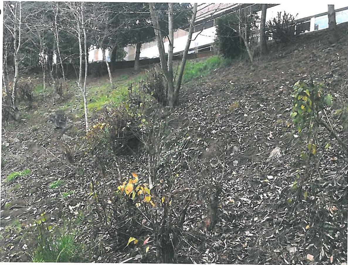
Photograph 1 – Looking northwest from base of slope looking west. Note the slumping area in foreground and potential outcrop of the Waverly Heights Basalt on the left side of the photograph.
