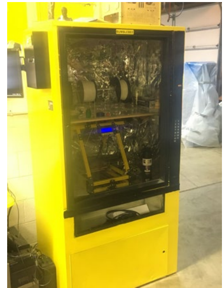
A 3D printer in the Knox Makers space, assembled inside of an old vending machine case.
