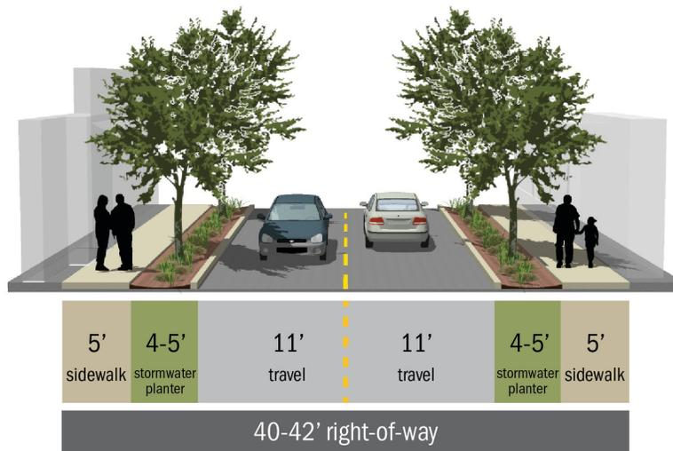
Figure A-12. Proposed Conceptual Cross-Section for Local Streets with a 40' right of way
