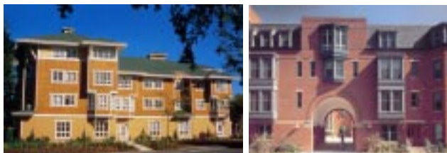
Recommended: Boldly articulated facades benefit from the inclusion of medallions, belt courses, varied cladding materials or other surface articulation (SW Yamhill and 4th, NW Hoyt and 12th, Oakland, CA, Boston, MA)
