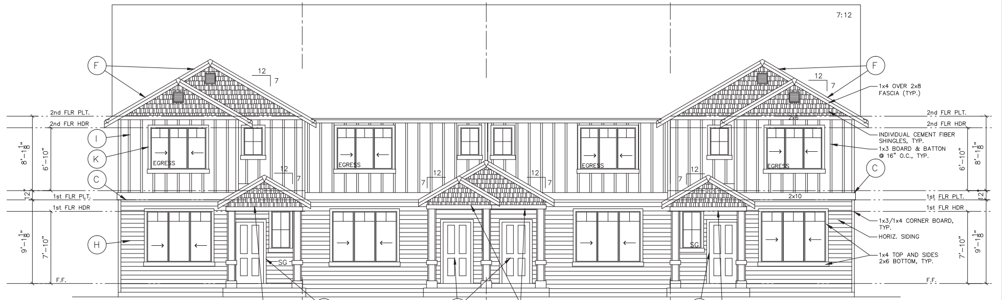
FRONT ELEVATION 4-PLEX BUILDING SCALE 3/16" = 1'-0"
