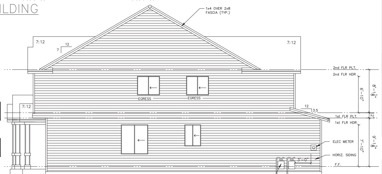
RIGHT ELEVATION 4-PLEX BUILDING SCALE 3/16" = 1'-0"
