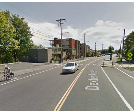
In the interim, streets can be re-channelized between existing curbs to begin the behavior change process as the City anticipates future roadways built out to the specifications. For example, Dexter Street, Seattle WA (before-after pictures above) include paint to delineate and channelize narrowed travel lanes in addition to bus stop bulb-outs and buffered bike lanes.
