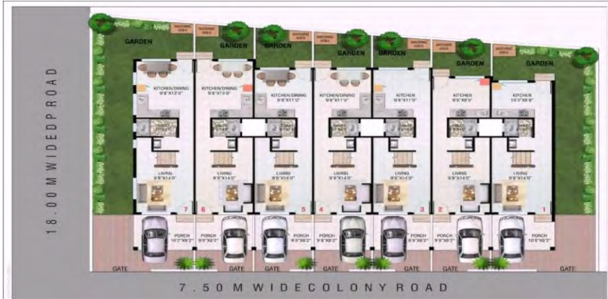
Figure 2: Site design example of a rowhouse development. Notice that each rowhouse is on their own lot, but still share walls.
